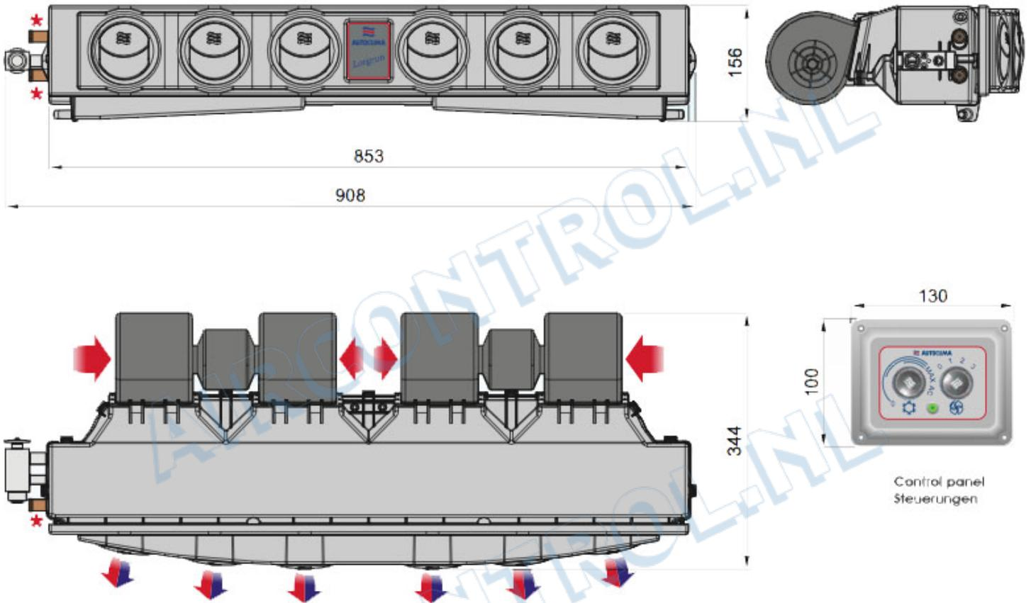
Evaporator studied specifically for conditioning big spaces in special vehicles. The control panel, equipped with thermostat and 3 speed selectors, allow a perfect regulation of the air. Also available with heating option (EH 75).
