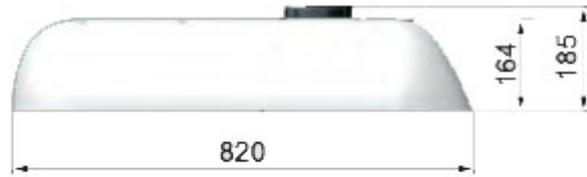
Roof top air conditioner expressly developed to condition medium size cabs and/or minibuses up to 10 seats. The reduced and compact dimensions make the installation easy and quick. Upon request are also available versions with heating (RTH 60).
