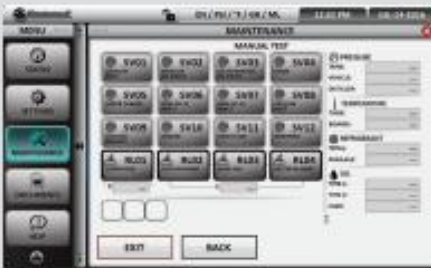
Maintenance Screen offered only to authorized service technicians allowing for quick and easy diagnosis
